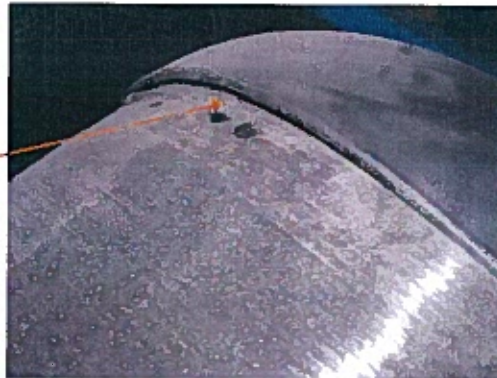
picture 6: loose protection cap
